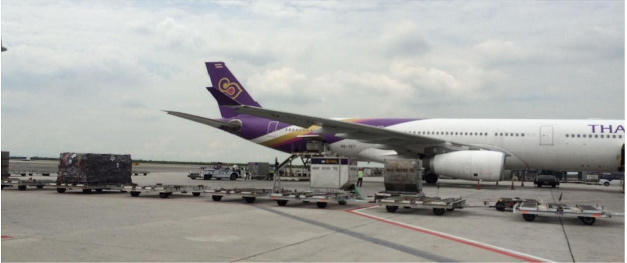
**Pallets and ULD's bound for loading onto a wide body aircraft**
